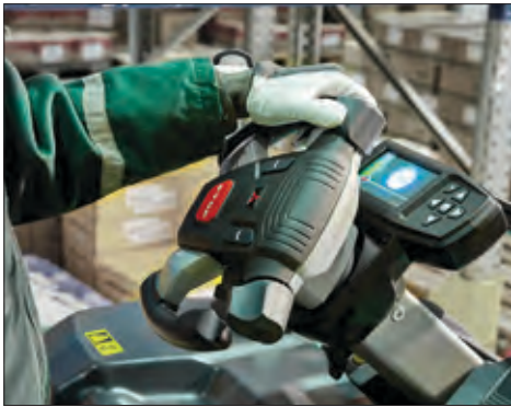
Multifunctional steering wheel with optional color display.
