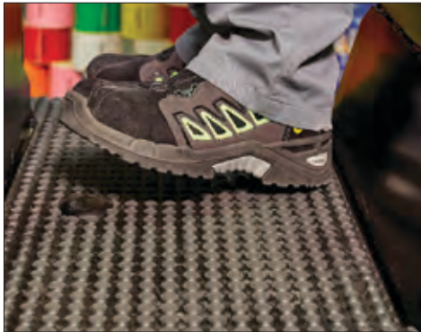
Foot switch for lowering the driver's platform.
